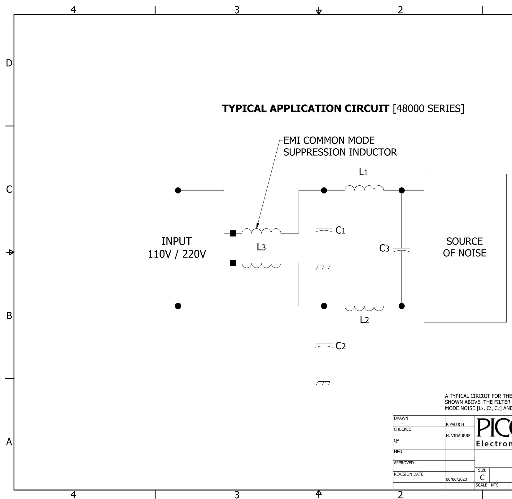
A TYPICAL CIRCUIT FOR THE ELIMINATION OF NOISE IS SHOWN ABOVE. THE FILTER CONTAINS TWO STAGES; ONE FOR COMMON MODE NOISE [L3, C1, C2] AND ONE FOR CONDUCED NOISE [L1, L2, C3]
